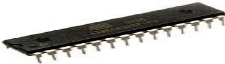
Fig. 6: ATmega328P in 28-pin narrow dual in-line package (DIP-28N)
