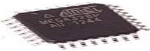
Fig. 7: ATmega328P in 32-pin thin quad flat pack (TQFP-32)
