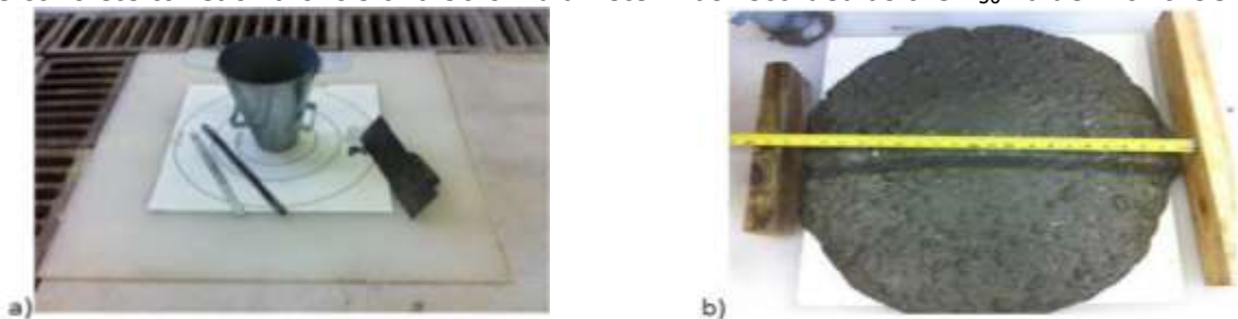
Figure 1 (a) Slump flow test set-up, (b) measuring slump flow of SCC mixture
